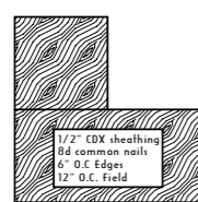
Min. Exterior Sheathing Required by Code = 3WP
